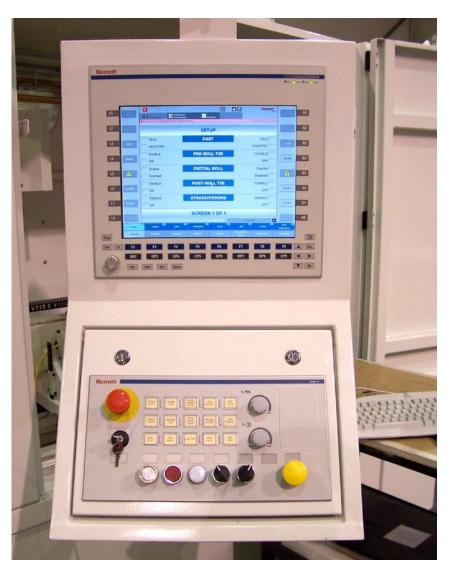
The installation uses a slim yet rugged Rexroth operator console connected with a single cable to the main electrical enclosure.
