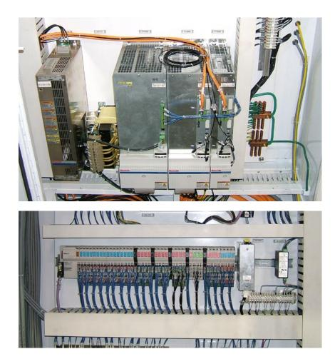
Ingersoll's machine takes advantage of distributed digital intelligent devices such as the IAC-R hydraulic valves, Fieldbus I/O, and electrical drives from Rexroth to significantly shrink panel space and wiring requirements.
