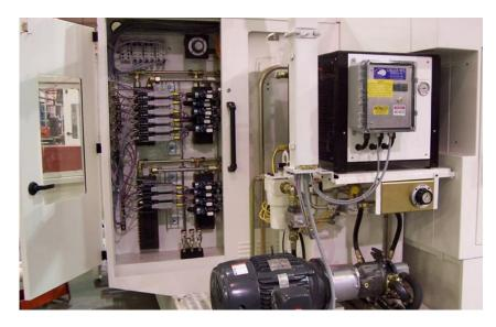
Using Rexroth IAC-R integrated axis controller proportional valves, Ingersoll CM Systems made its machine 25 percent more compact.
