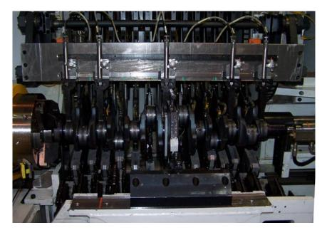
Depending on the crankshaft requirements, the rolling machine includes from nine to 13 arms of independent rolling axes.
